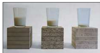
MDF 74 ml/dm 3 Span 46 ml/dm 3 SWL STAB 11 ml/dm 3
